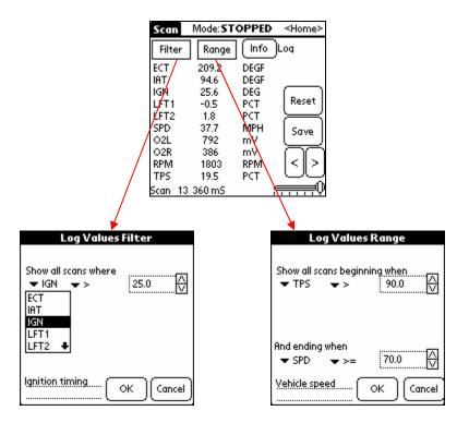
Pick a parameter from the drop-down list, pick a condition, then enter a value. In the example on the left, all scans will be shown that contain ignition timing advance greater than 25 degrees. In the example on the right, scans will be filtered starting when the throttle is over 90% open and stopping when the SPD reaches 70 mph.
